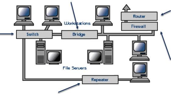
A repeater boosts the signals to strengthen what is lost during data transferring. The signal is electronically amplified.
