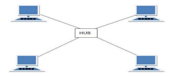
To allow direct data traffic between the hub and the machine, a "star topology" is proposed to handle this structure.
