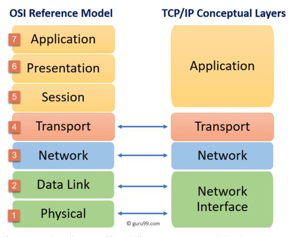
TCP/IP (TCP stands for Transmission Control Protocol and IP stands for Internet Protocol) model is the central intelligence system to determine how the computer speaks with the internet. It is specially designed to provide reliable internet services.
