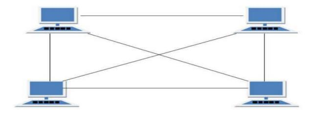
The third candidate is the "mesh topology" which links one machine with another.
