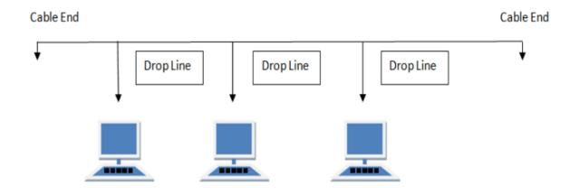
The most foundational structure is the "bus topology". There is one main cable from the beginning to the end where each machine is dropped out as a branch.
